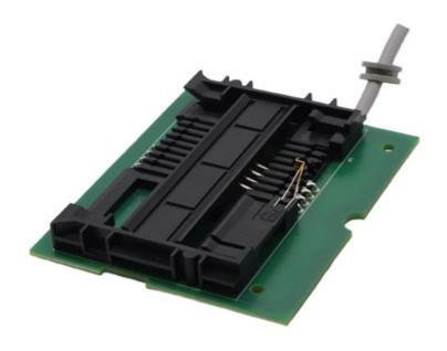
The Omnikey 5122 reader board from HID is a dual interface USB 2.0 smartcard reader that reads/writes to both 13.56 MHz contactless smartcards and virtually any contact smartcard technology.
